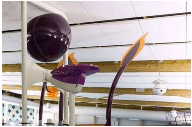
b. Quietspace® Panels with gaps to keep the roof cavity well-ventilated
